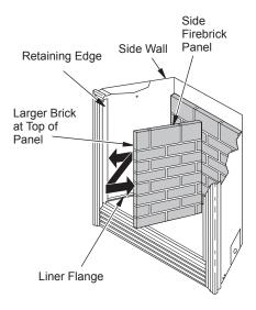
Figure 4 - Placing Side Firebrick Panel Behind Retaining Edge
